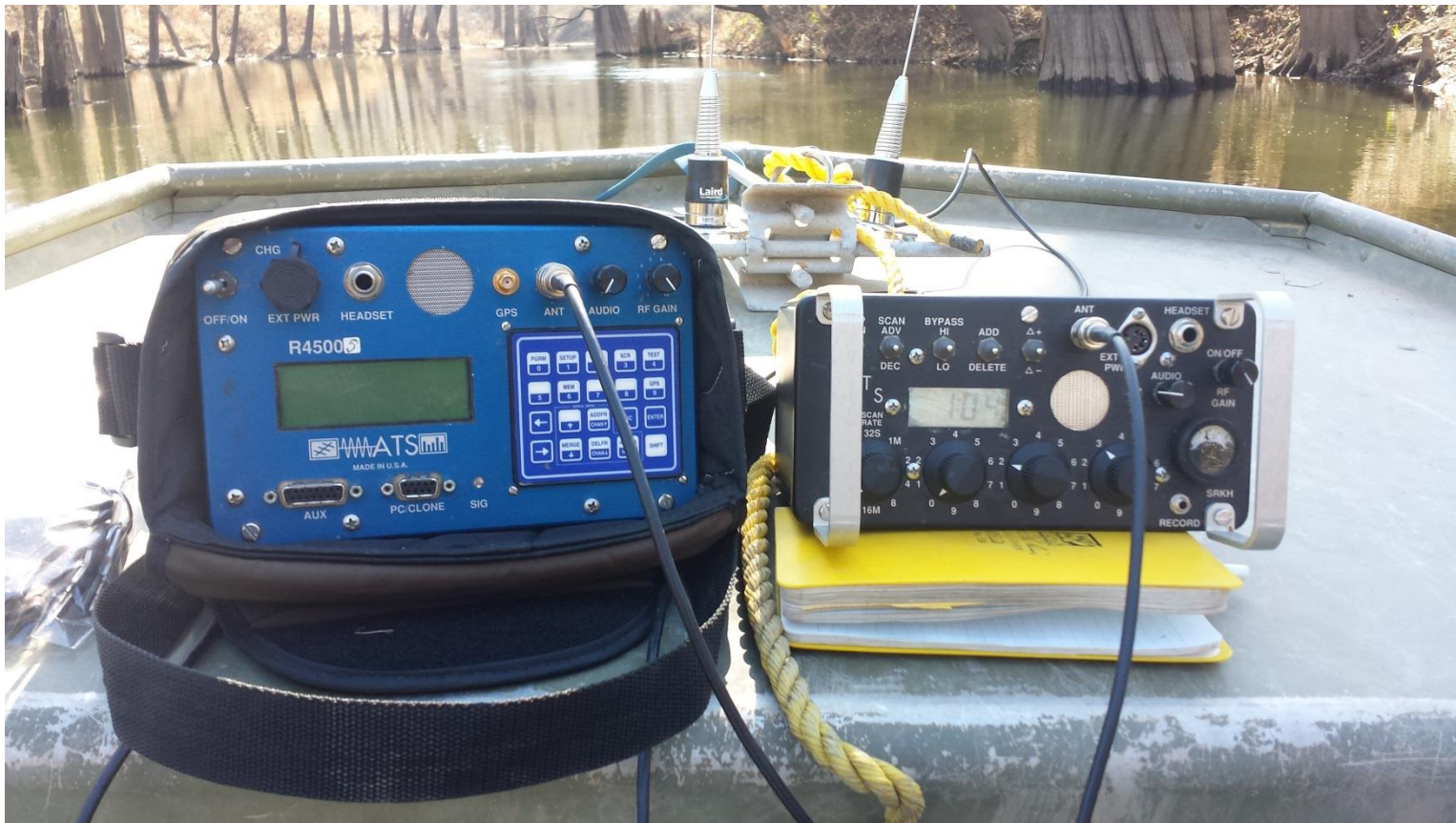
Figure 22. Typical radio receiver configuration for boat tracking. Two receivers running concurrently to reduce the chance of passing tagged fish as the radios scan through the 47 tag numbers.
